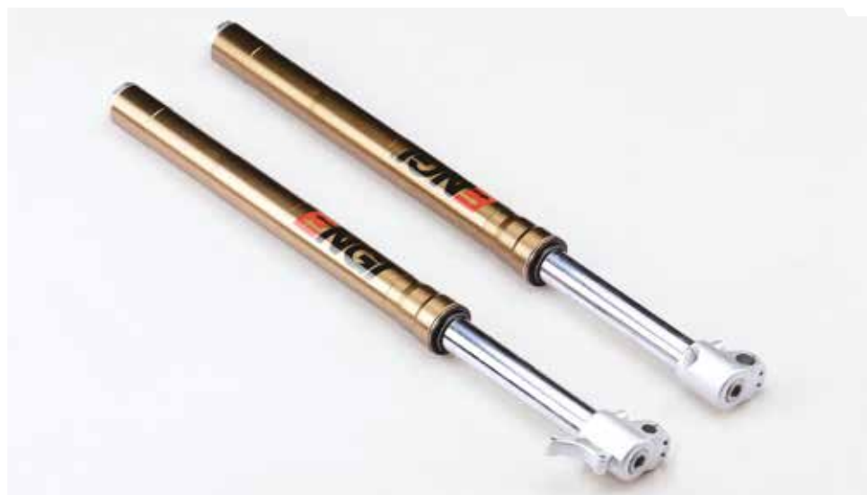
FOURCHE ENG1® RÉGLABLE COMPRESSION DÉTENTE ENG1® FORK WITH ADJUSTABLE COMPRESSION & REBOUND
